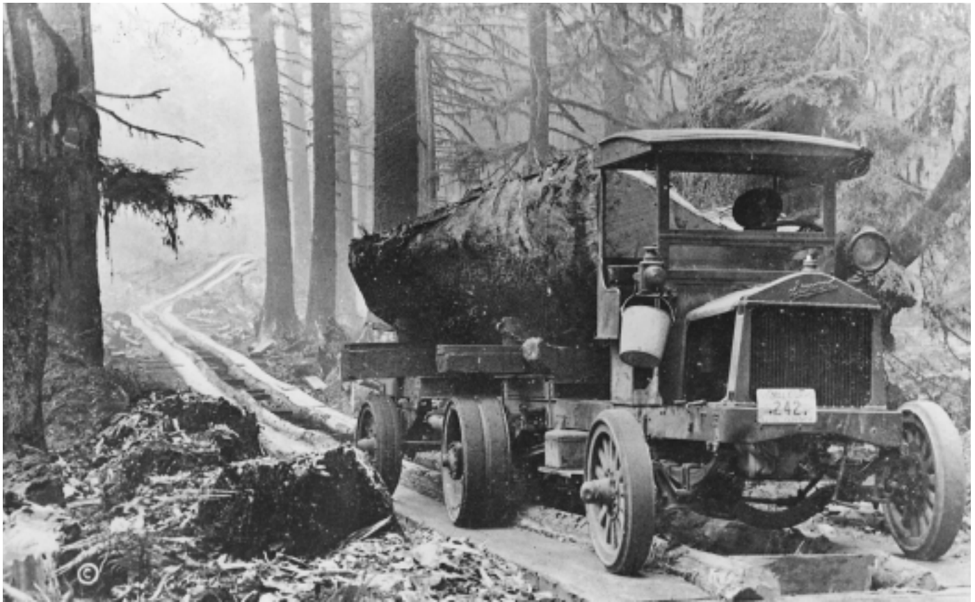
This army truck hauls a rived spruce log over the hand-built plank road.
